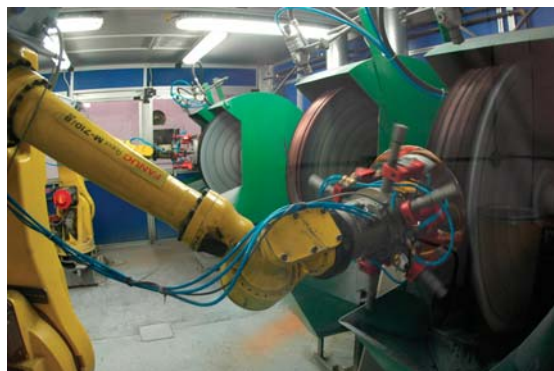
But buffing cymbals to a gleaming finish is performed by a team of computer-controlled robot arms.
