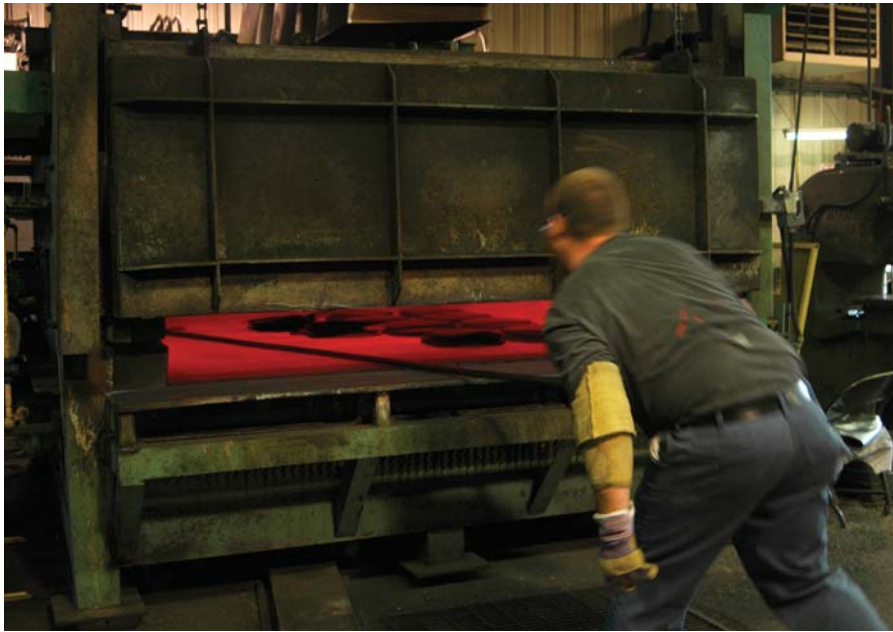
Where it all begins. Disks of a special bronze alloy are heated prior to being rolled into cymbal blanks.
